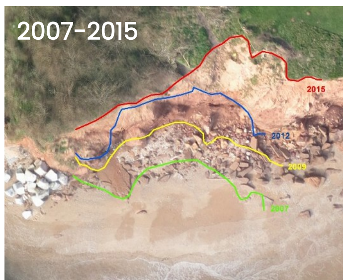
Figure 1 Aerial imagery of Sidmouth displaying cliff erosion lines, from the years 2007, 2009, 2012, and 2015.
