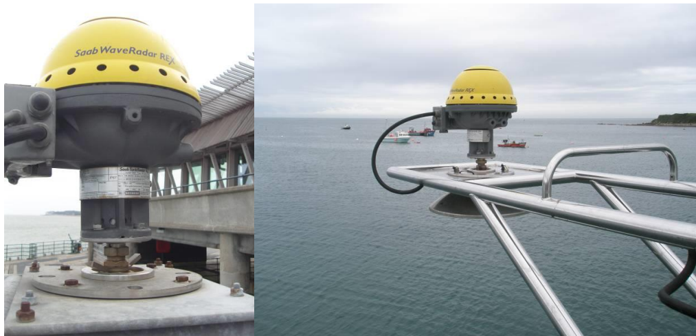
Figure 1: WaveRadar REX at Deal Pier (left) and Sandown Pier (right). Photos courtesy of Fugro GB Marine Limited.
